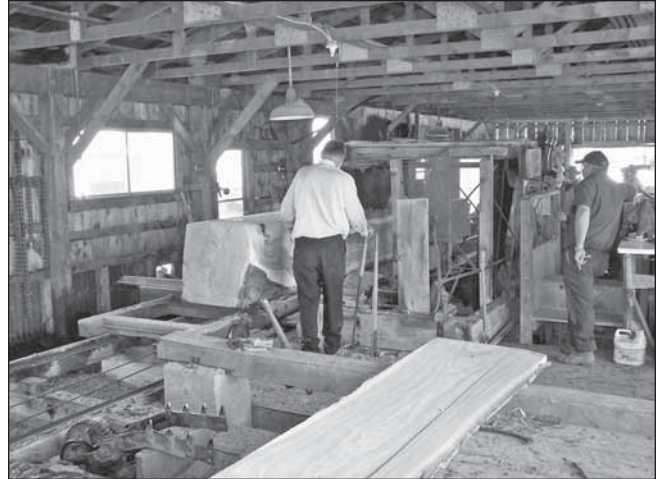
Searson Saw Mill, Watford, 2007: Carlyle Searson is operating a steam-powered saw, using scrap wood as fuel for the engine.
