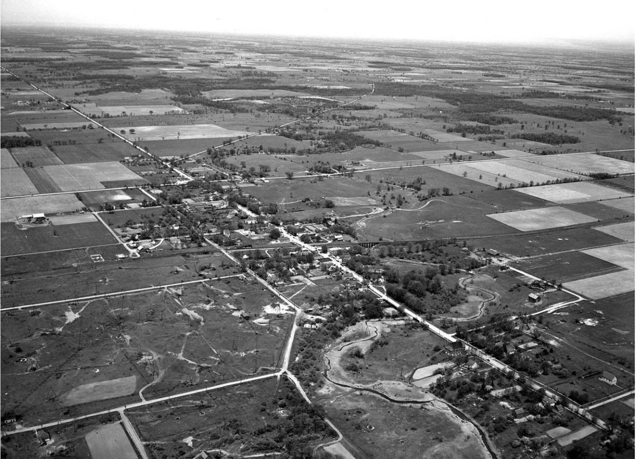
Note: The Plank Road angles off to the right at the far end of town. The railway bridge is visible at the edge of town on the right. The oil field with its powerhouses and jerker lines fills the lower-left of the photo.
