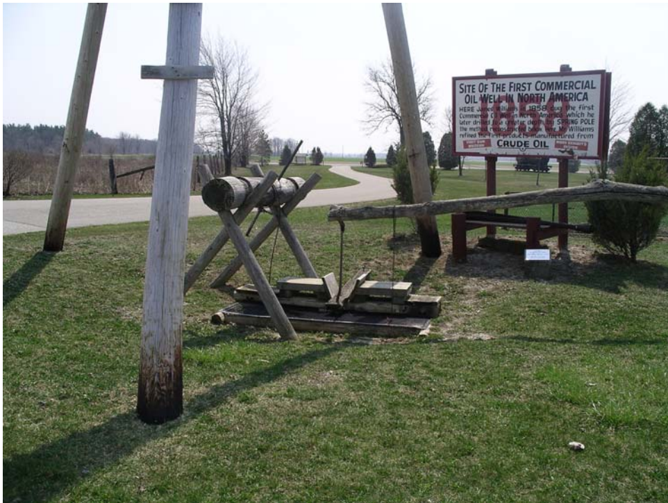
Figure 8. Williams-dug oil well near the museum with a three-pole derrick – Oil Springs. (A. Roos, Parks Canada, April 2005)
