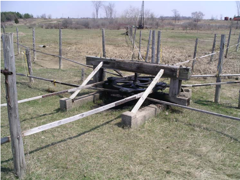
Figure 10. Spider wheel allowing changes of direction of jerker line, with a contemporary derrick in the background – Oil Springs. ( A. Roos, Parks Canada, April 2005 )
