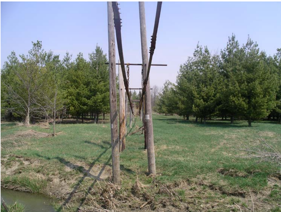
Figure 11. Jerker line coming down a hill and over a creek – Oil Springs. ( A. Roos, Parks Canada, April 2005 )
